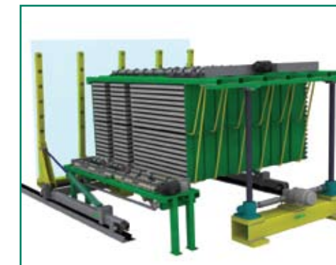
Storage Rack raised to receive remnant from the cutter
