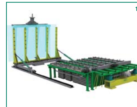
Tilt Arms traversing to retrieve glass from the crane glass grab
